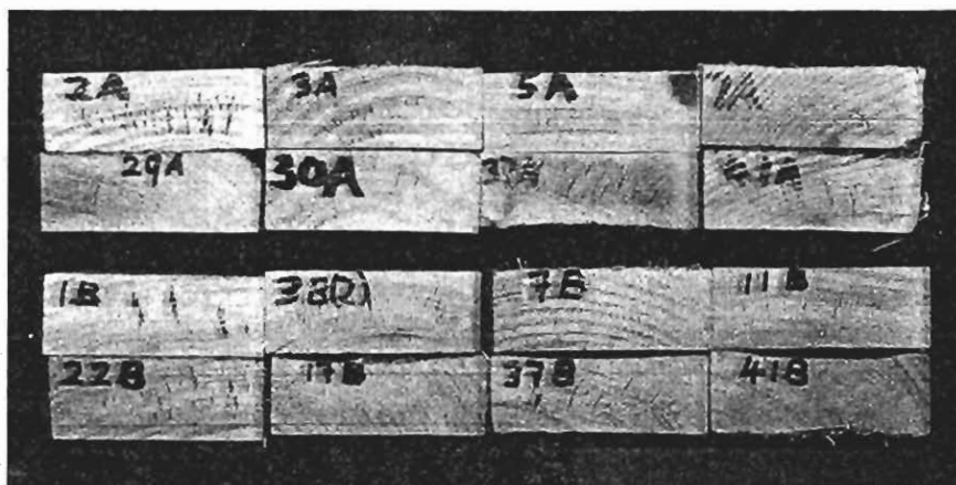
Absence of internal checking in Victorian ash when kiln drying is delayed until the core moisture content is below fibre saturation point. The two upper rows were dried at 120°C DBT/70°C WBT and the two lower ones at 70°C DBT/60°C WBT.
